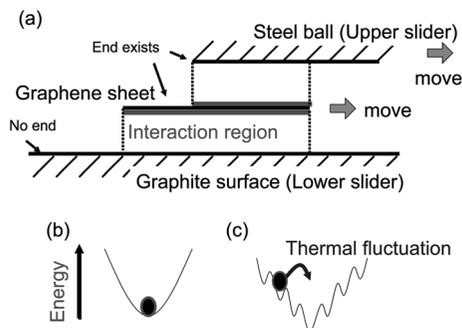
**Fig. 9** A conceptual illustration of the end effect.
